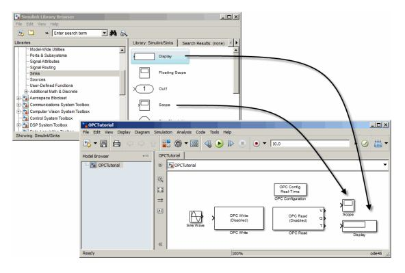
and place it above and to the right of the OPC Read block. Also drag a Display block into the Simulink Editor and place it below the Scope block.
