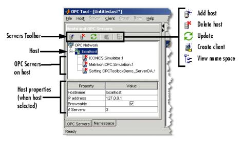
Note that the local host in this example provides three OPC servers. The Server ID for this example is 'Matrikon.OPC.Simulation.1'.
