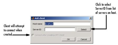
When you supply a hostname, you will be able to select the Server ID from a list, by clicking **Select**. Using the Add client dialog, you can also automatically attempt to connect to the server when the client is created, by checking **Connect after creating OPC Client** before clicking **OK**.
