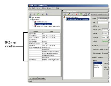
The OPC server properties include diagnostic information, such as the supported OPC Data Access interfaces, the time the server was started, and the current server status.
